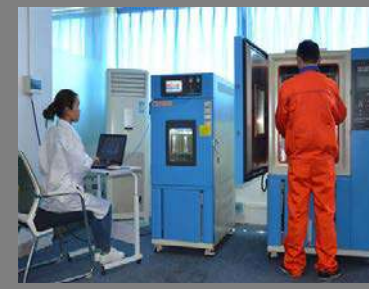
Temperature/Humidity Cycle Test
